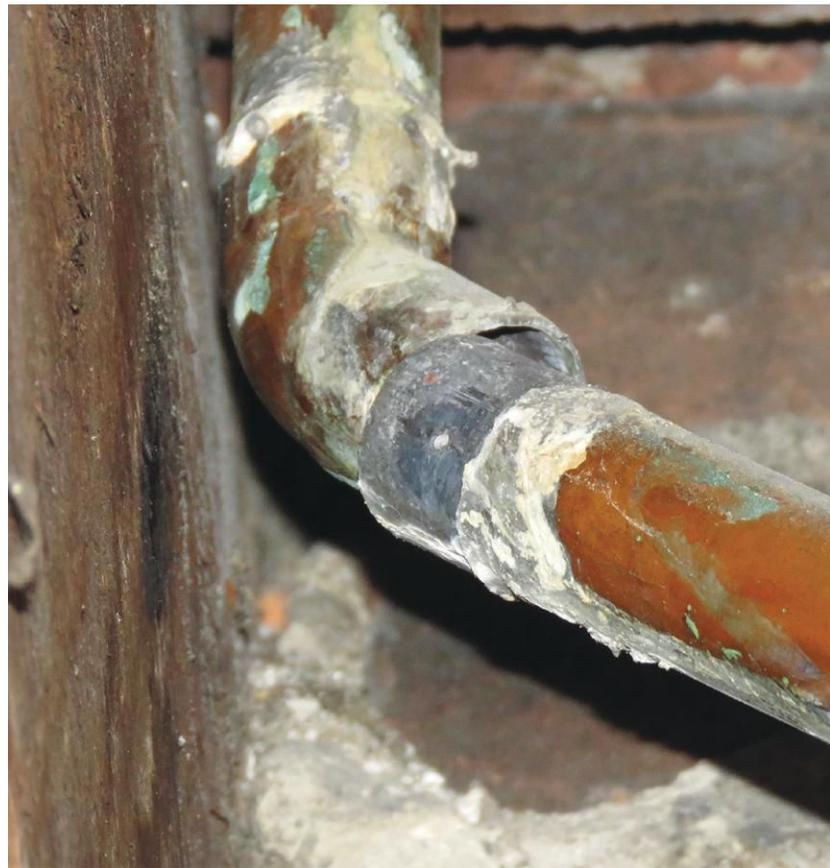
curs after the ice plug melts and the water begins to flow. Thawing conditions typically occur when the outside temperature is at or above 35°. When the ice plug melts and the water supply is not isolated, the water will flow out of the break until such a time that the leak is identified and isolated. In some cases, such as when buildings are vacant, this duration may be months.
